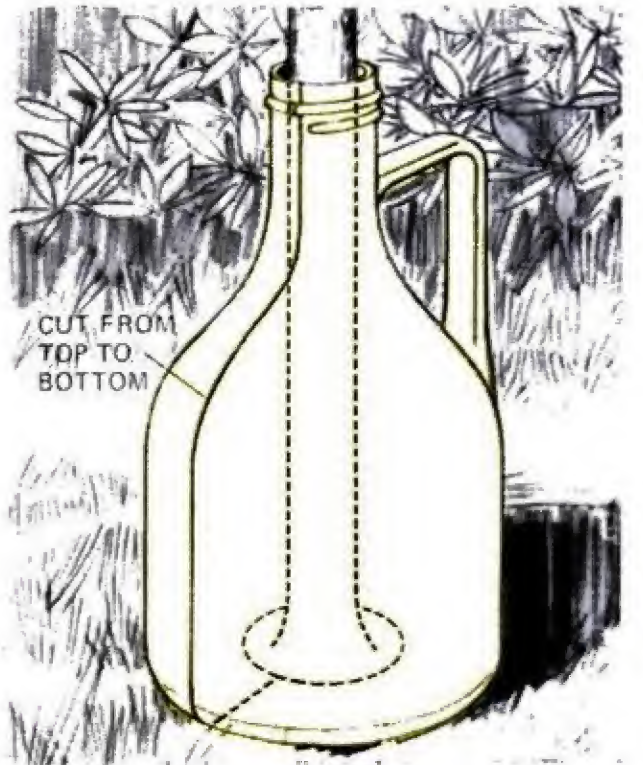
GALLON PLASTIC BOTTLES can be used to protect small trees from rodent damage. Just cut a hole in the center of the bottom, make a slit down the side and put in place.— Ralph O. Fritts, Amsterdam, Mo.
